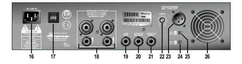
**16. AC LINE IN:** Firmly insert the female end of the supplied AC power cord into this socket. The grounded power cord should only be plugged into a grounded power outlet that meets all applicable electrical codes and is compatible with the voltage, power, and frequency requirements stated on the rear panel. **Do not attempt to defeat the safety ground connection.**
